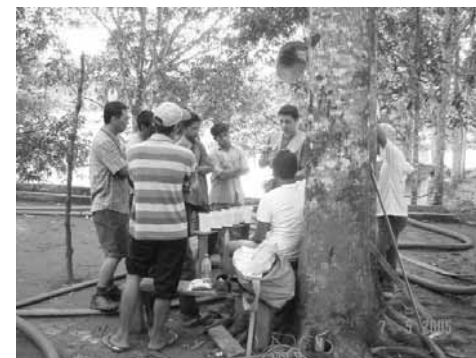
Figure 2: Operator training on simplified jar-test procedures for coagulant dose determination.
